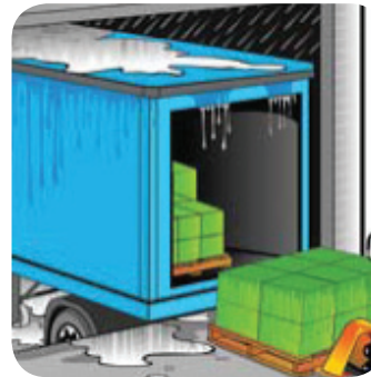
Water infiltration onto the loading dock area can lead to wet and slippery floors which can be dangerous to personnel.
