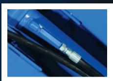
The inverted deck cylinder is continually self-bleeding, reducing internal corrosion and increasing velocity fuse efficiency.
