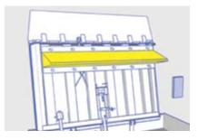
The optional foam draft pad provides additional sealing against outside elements and enables better environmental control.
