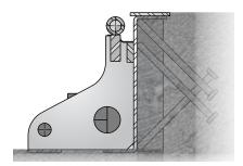
Full rear frame is embedded into concrete, enabling a robust installation and improving the dock's rear support.
